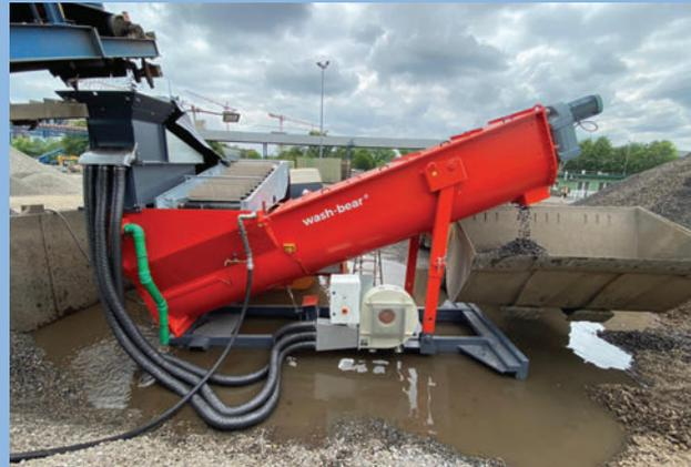
optional) 'clean extension', the wash-bear® becomes a powerful wet-processing system for the removal of fine fractions, e.g. when washing track ballast.
